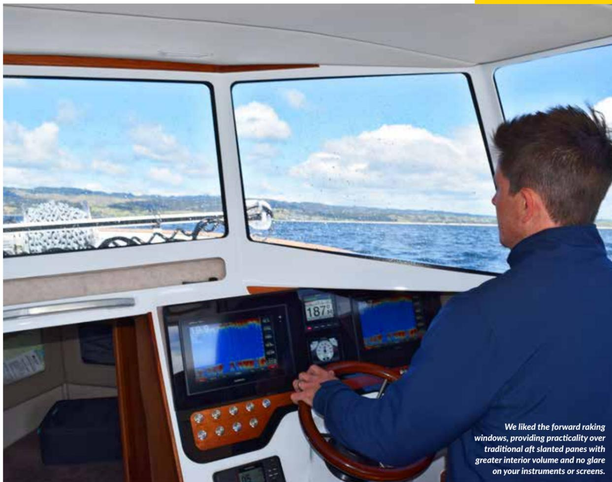
We liked the forward raking windows, providing practicality over traditional aft slanted panes with greater interior volume and no glare on your instruments or screens.
